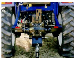
For the three-point hitch, we use the Category II connector up to the international standard. Meanwhile, enhanced lifting arms and quick-attaching connectors improve the general strength on the basis of matching various implements.
