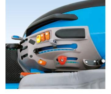
**TWO-SPEED PTO WITH MODULATED ENGAGEMENT** The PTO offers two speeds: 540/540e rpm (standard) or 540/1000 rpm (option). An electrohydraulic push button control, standard on all models, enables smooth and modulated engagement of the PTO, ensuring a soft start-up of the implement.
