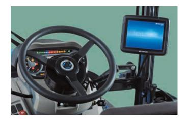
**ELECTRONIC STEERING WHEEL** The electronic steering wheel, via the touch screen monitor, allows precise steering during row-crop operations with a maximum error of 2 cm.
