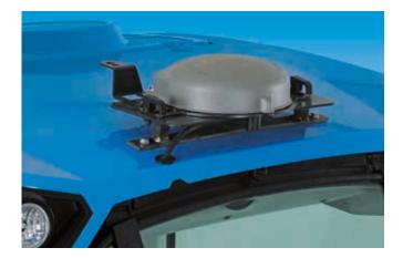
**SATELLITE ANTENNA** The satellite antenna placed on the cab roof receives the GPS signal.
