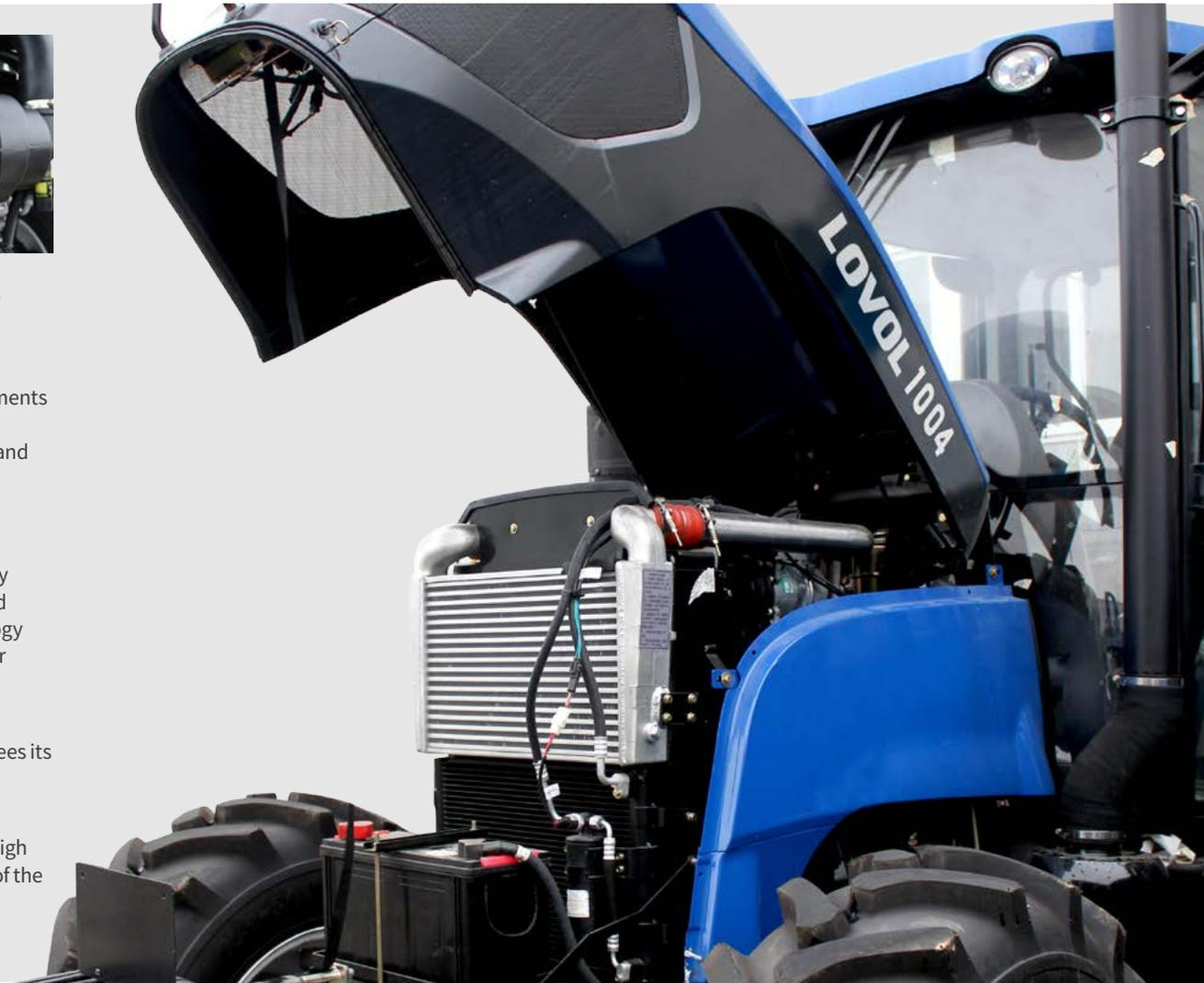
Standard Lovol engine: Cylinder number: 4; Displacement: 4L; Engine power: 66-80 kW (80-100Hp); PTO power: 56-68kW; Rated speed: 2,200; Intake mode: natural intake.
