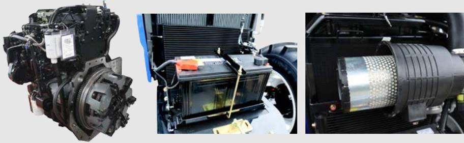
Lovol engine is equipped with the well-known European engine technology, four-cylinder engine dual-valve design, and turbocharged air inlet system.
