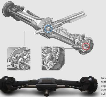
New design front axle with bigger burden capacity, higher clearance, two steering cylinders structure
