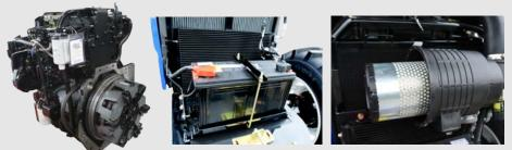
Lovol engine is equipped with the well-known European engine technology, four-cylinder engine dual-valve design, and turbocharged air inlet system.
