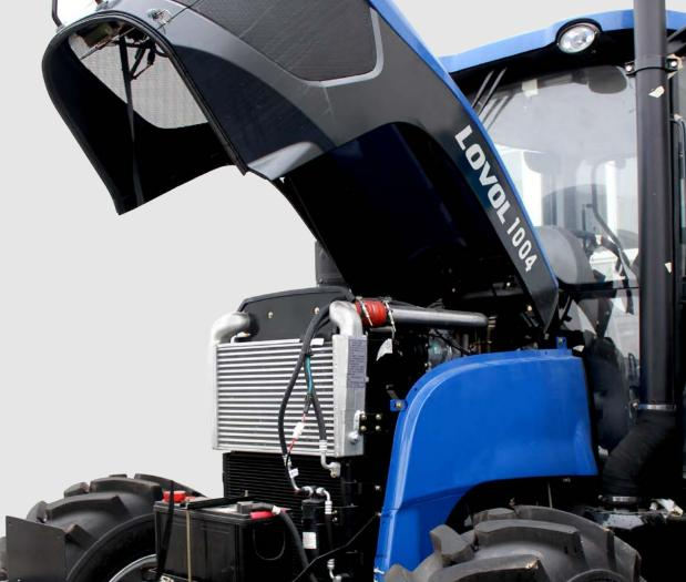
Standard Lovol engine: Cylinder number: 4; Displacement: 4L; Engine power: 66-80 kW (80-100Hp); PTO power: 56-68kW; Rated speed: 2,200; Intake mode: natural intake.
